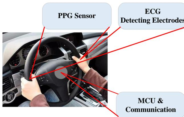
Fig. 1. Scenario of the real time monitoring of car driver's system. drivers' bio-data such as ECG, PPG, blood pressure and blood oxygen saturation. Moreover, this system will connect to cloud server through mobile internet, return drivers' bio-data back to monitor center, to secure each drivers' and passengers' safety.
