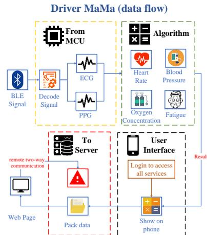
Fig. 6. System block of data side.
