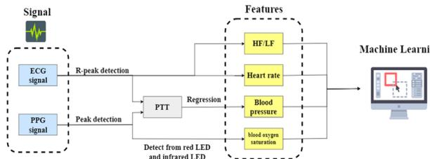
Fig. 7. System block of algorithm
