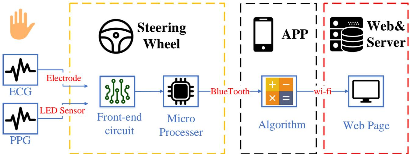
Fig. 2. System block of wireless bio-signal acquisition and application.
