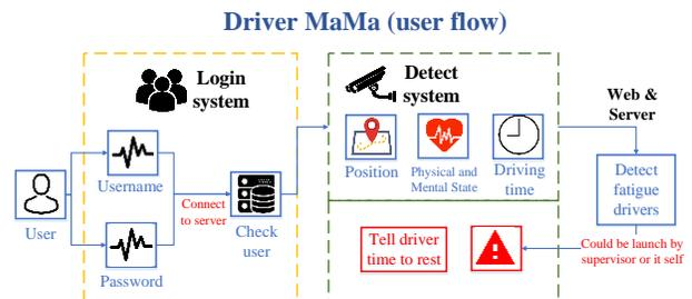
Fig. 5. System block of user side.
