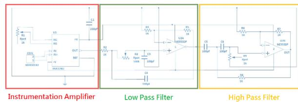
Fig. 4. Front-end circuit structure.
