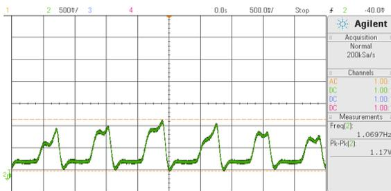
Fig. 11. The waveform of PPG signal.
